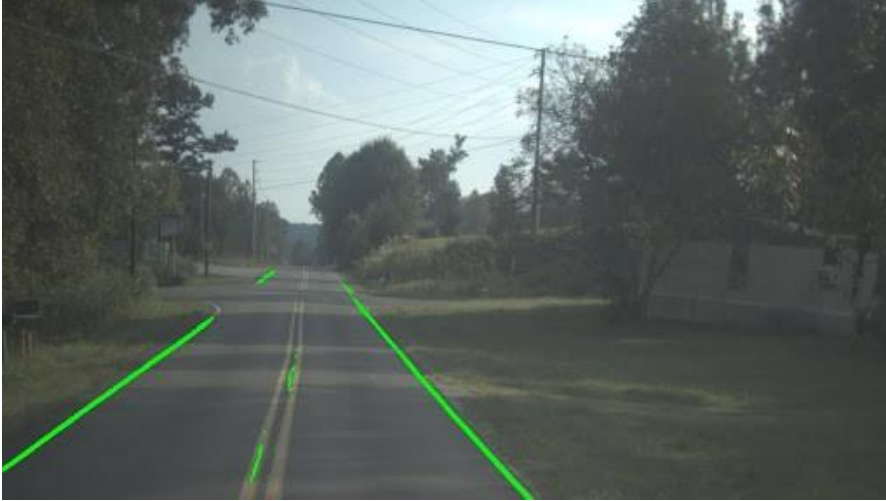
Fig. 5 An example image with lane markings segmented by our fine-tuned SegFormer model, overlaid on the original image
