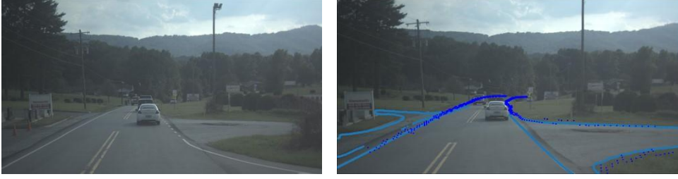
Fig. 6 Filtered and integrated road edge segmentation result (right) of an example image (left), where the filtered and integrated road edge segmentation pixels are shown in light blue, and projected LiDAR road edge pixels are shown in dark blue.
